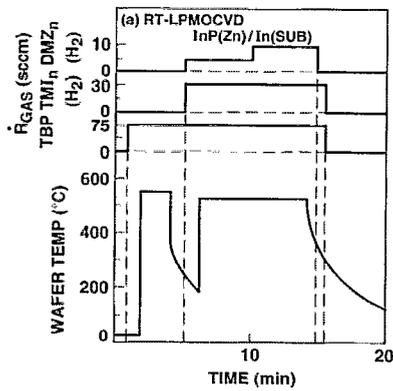
FIG. 1. Schematic process flow chart of a RT-LPMOCVD Zn-doped InP layer (100 thick).
