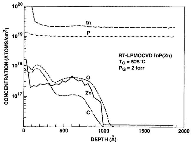
FIG. 4. SIMS depth profile of Zn-doped RT-LPMOCVD InP layer grown on SI-InP substrate at 525 °C for 2 min.
