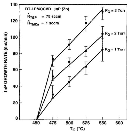
FIG. 5. RT-LPMOCVD Zn-doped InP layer growth rate as a function of the growth temperature and the chamber pressure.
