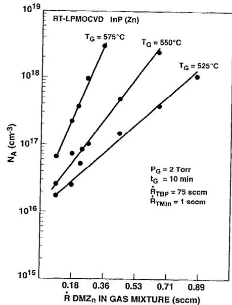
FIG. 3. Carrier concentration ( $N_A$ ) at Zn-doped RT-LPMOCVD InP layer, as a function of the DMZn flow rate and the growth temperature.
