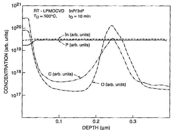
FIG. 4. SIMS depth profile of an undoped RT-LPMOCVD InP layer grown onto SI-InP substrate at 500 °C for 10 min.
