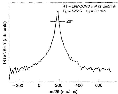
FIG. 2. Double crystal x-ray diffractometry of an undoped RT-LPMOCVD InP layer grown on SI-InP substrate at 500 °C for 10 min.
