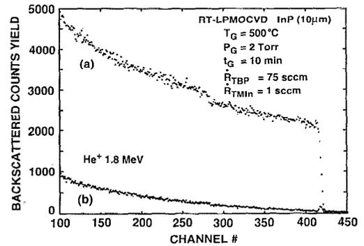
FIG. 3. RBS of an undoped RT-LPMOCVD InP layer grown at 500 °C for 10 min, both at rotating direction (a) and along  $\langle 100 \rangle$  lattice axis (b).
